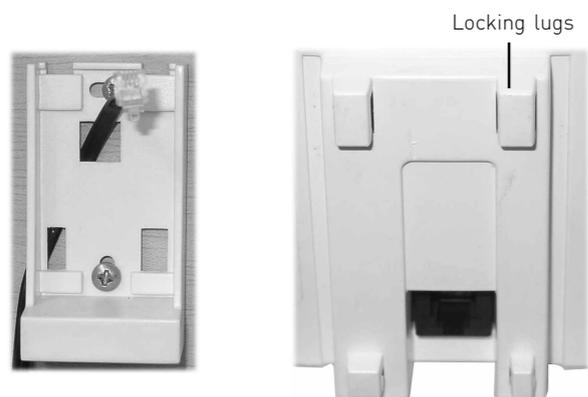
To remove the repeater from the wall, insert a screwdriver between the front lip of the bracket and the repeater, and lightly push the repeater upward.
